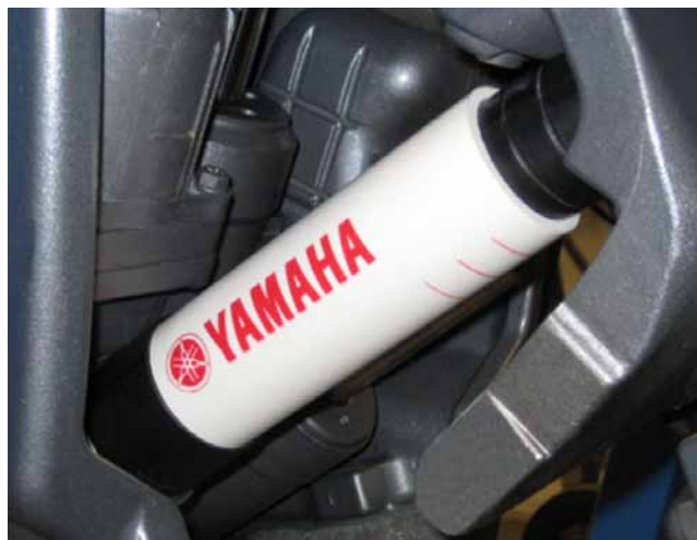
Another transom-saving device is a tube like the one pictured above that absorbs the weight of the outboard, rather than letting the weight fall directly onto the transom.
