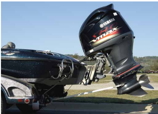
One way to protect your boat's transom during trailering is to install an adjustable bar to support it.
